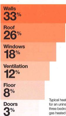
Typical heat loss for an uninsulated three bedroom gas heated semi-detached home.
